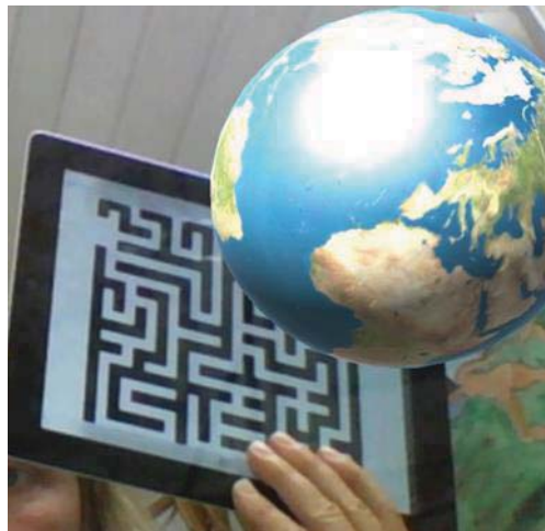
Figure 4: Image-based AR. The black and white image enables the virtual 3D Earth
