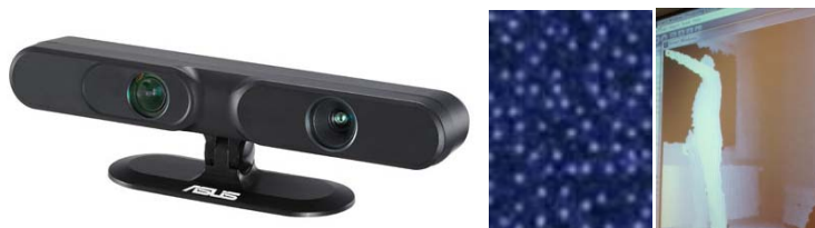
Figure 1. (a)The open platform Asus Xtion Pro (Asus, 2013); (b) IR Projected light on a blank surface; (c) 3D image based on IR information
