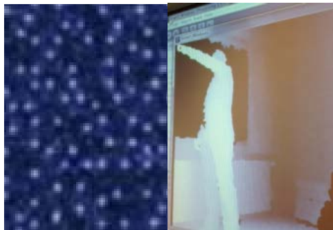
Figure 2. (a) IR Projected light on a blank surface; (b) 3D image based on IR information
